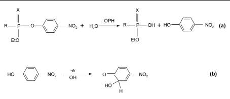
Scheme 2 (A) Reaction scheme of the OPH catalyzed hydrolysis of parathion, methyl parathion and paraoxon. (B) Electrochemical oxidation of *p*-nitrophenol. Parathion: X = S, R = ethoxy; methyl parathion: X = S, R = methoxy; paraoxon: X = O, R = ethoxy
