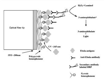
**Fig. 5** The biosensor scheme describing the various steps involved in the immunoassay using ITO–poly(pyrrole-benzophenone)-coated optical fibers for the detection of anti-Ebola virus in sera samples.<sup>121</sup>
