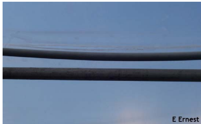
One of numerous large holes where the conduit touches the greenhouse film.
