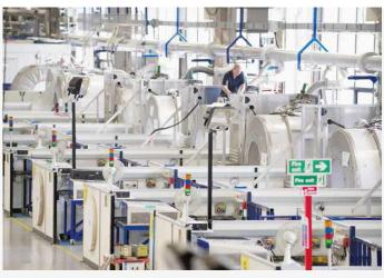
7T magnet volume-production at Siemens Magnet Technology, Oxford, UK – thanks to over 30 years of engineering skills and well-founded process expertise in building magnets for 1.5T and 3T.
