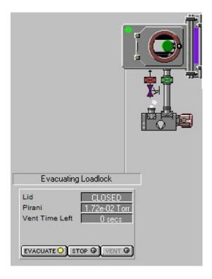
The Vent Time Left feedback will start counting down. When the loadlock reaches atmosphere and the Vent Time Left is 0 secs, open the loadlock lid and place your samples on the 6" Si wafer carrier in the loadlock. Verify that the 6" Si wafer carrier flat is right against two screw stops (adjust as needed). Close the lid and pump the chamber down by pressing **STOP** and then **EVACUATE**. Enter the wafer ID and click OK. When the Green dot appears, it indicate it is ready to run the process.
