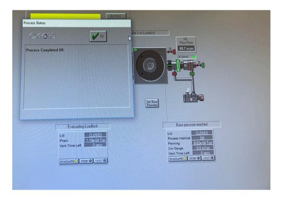
Click ok, the wafer will be returned to the loadlock automatically for removal.
