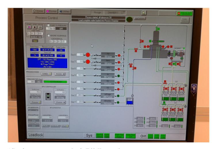
Adjust the process temperature using the Table Heater setting.
