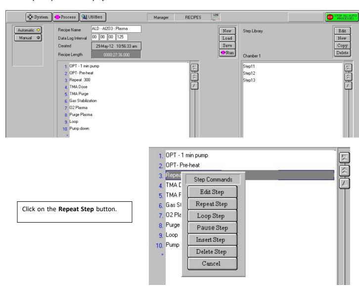
Enter the number of cycles you require for the desired film thickness.
