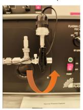
To vent the chamber, turn the black handle of the 3-way valve so that its arrow end points to the right.
