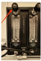
Slightly adjust the **metering valve** (1/8 of a turn or less) and allow the pressure to stabilize at 600 mTorr.
