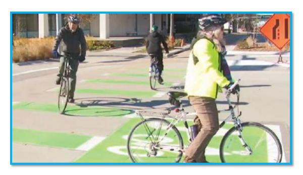
IMAGE 20: Example of painted boxes as an additional measure of safety and priority for cyclists. 116
