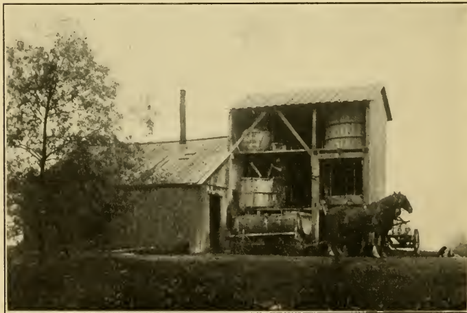
FIG. 251.—Plant for making lime-sulphur solution in large quantities. (Photo. Ohio Exp. Sta.)
