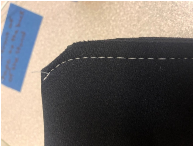
Figure 7. Neoprene piece with seam allowance trimmed.
