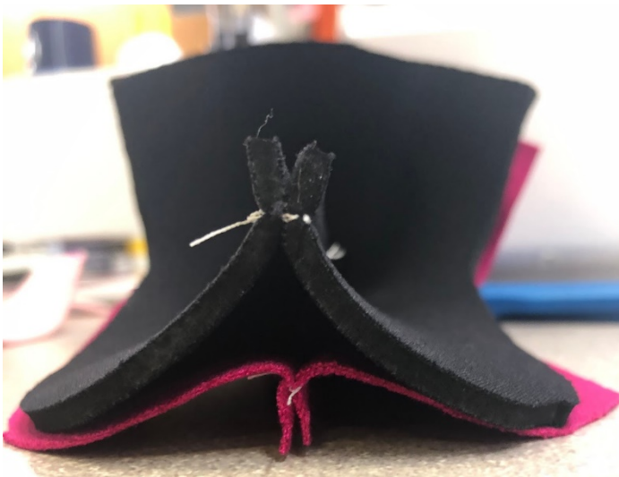
Figure 8. Neoprene and Ponte de Rome Fabric pieces pinned together. See video
