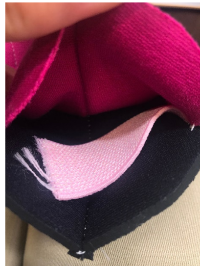
Figure 9. Elastic sandwiched between fabric pieces.
