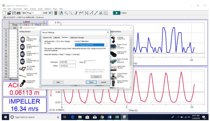
Figure A31. LoggerPro screenshot showing options for setting up sensors – equations tab (ONLY IF NEEDED).
