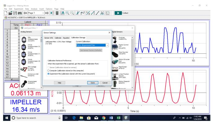
*Figure A32. LoggerPro screenshot showing options for setting up sensors – calibration storage (ONLY IF NEEDED).*
