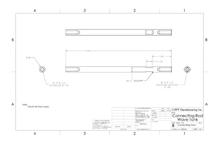
Figure A20. Snapshot of CAD drawing for the linkage arm. A PDF version of the file is available upon request.
