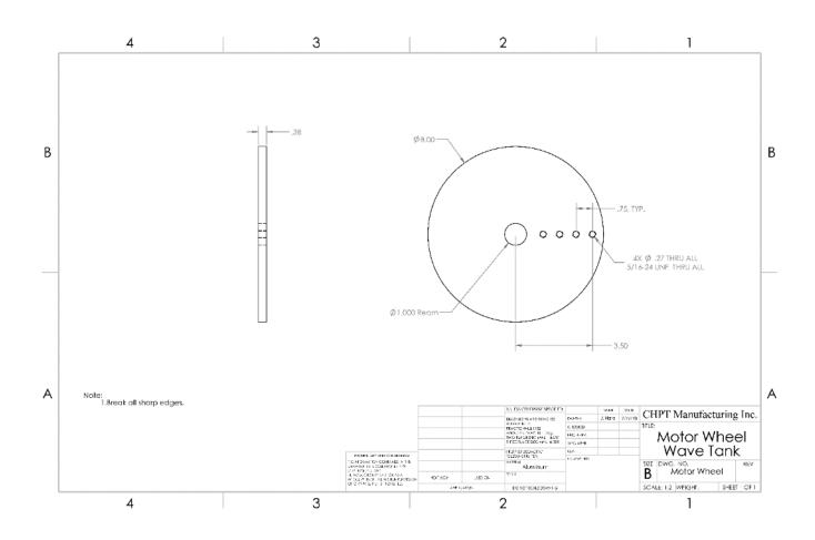
*Figure A19. Snapshot of CAD drawing for the motor wheel. A PDF version of the file is available upon request.*
