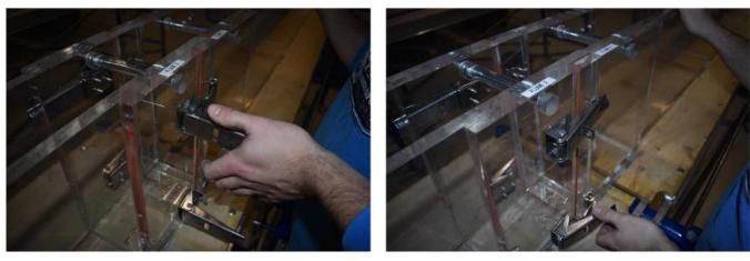
*Figure A9. Pictures showing mating of flume halves and adjustment and closing of draw latches.*
