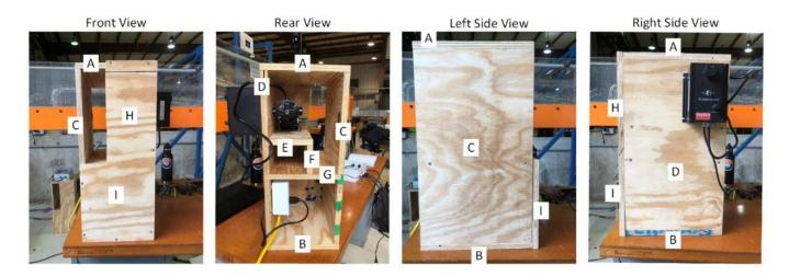
*Figure A36. Completed motor stand assembly from different views. Letters correspond to pieces shown in Figure A35.*
