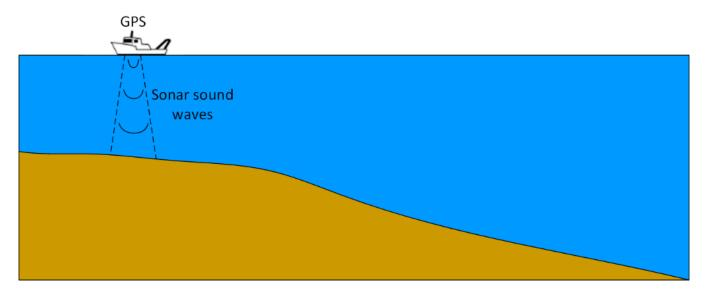
Figure 11. Schematic showing a survey vessel with GPS and sonar device for offshore beach profile measurements.
