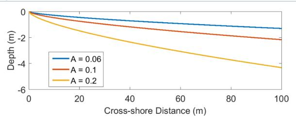
*Figure 13. Example equilibrium beach profiles for different profile scale parameters.*
