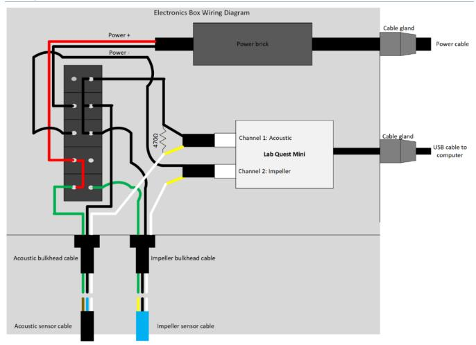
Figure A34. A wiring diagram for the electronics box.
