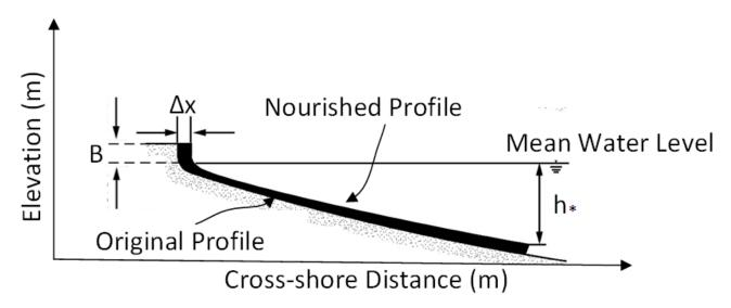
Figure 21. Schematic showing the original beach profile and the nourished beach profile providing the additional dry beach width,  $\Delta x$ .
