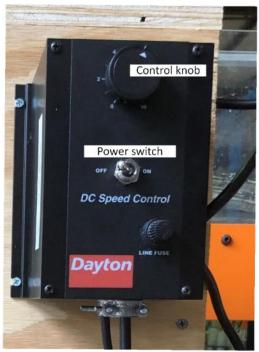
*Figure A16. DC controller showing power switch and speed control knob.*
