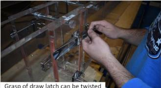
Grasp of draw latch can be twisted to increase or decrease tension when latch is closed
