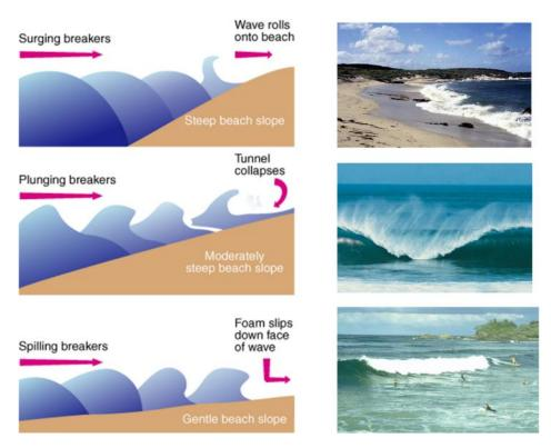
Figure 14. Schematic and associated image of different breaker types related to beach slope.
