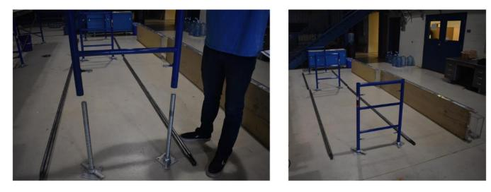
Figure A1. Pictures showing frame stands and jack screw set up.
