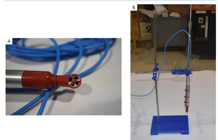
Figure A24. A) Close up view of the Omni Instruments Impeller Current Meter. B) The impeller attached via cable ties to a ¼" diameter stainless steel tube and affixed in the lab stand.
