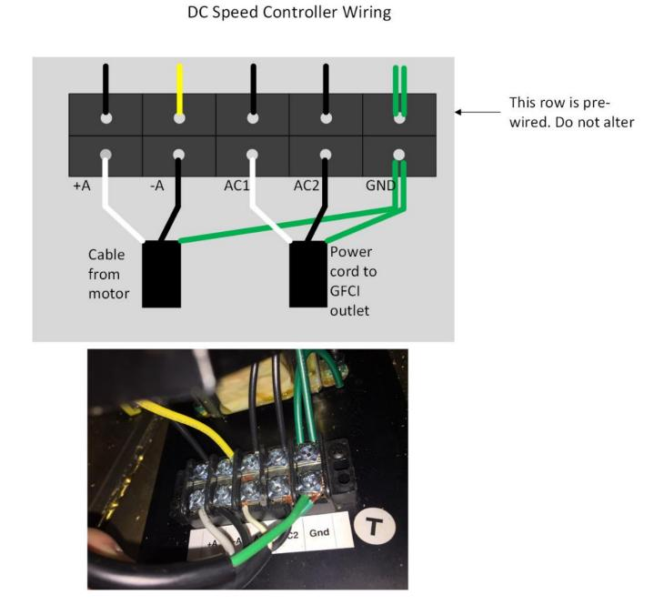
*Figure A37. Wiring diagram and picture showing the wiring inside the DC speed controller.*
