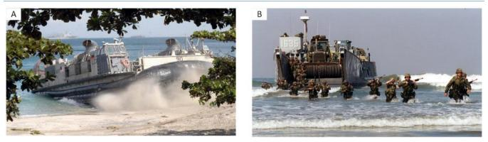
Figure 15. A) Landing Craft Air Cushion (LCAC) approaching a steep beach face. B) Military personnel exiting a landing craft that was restricted from farther landward motion due to the shallow beach slope.
