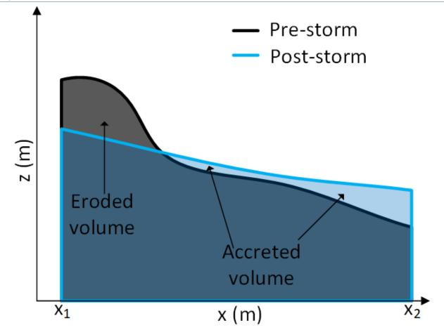
Figure 17. Schematic showing the areas under the curve determined through integration and eroded and accreted volumes from pre- and post-storm measurements.
