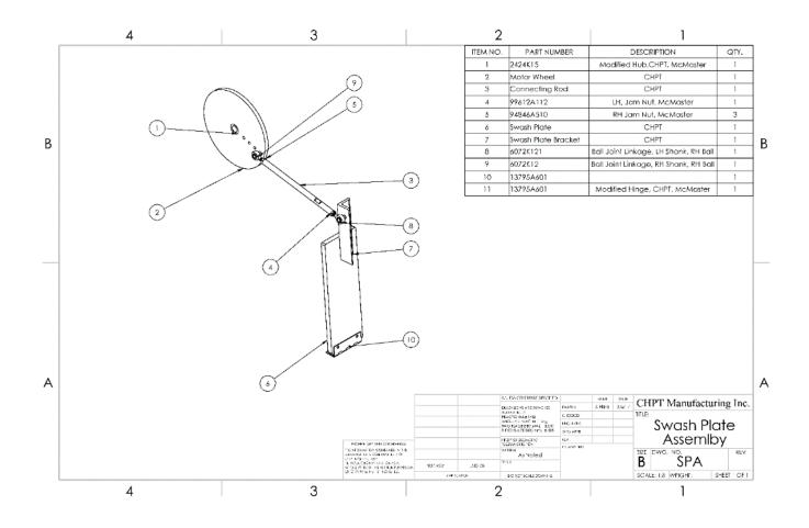
*Figure A18. Snapshot of CAD drawing for the wave paddle and motor wheel. A PDF version of the file is available upon request.*
