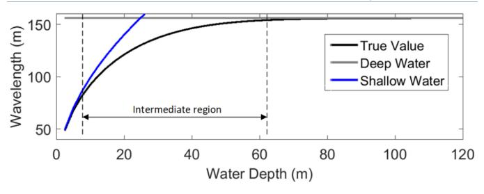
Figure 4. Wavelength as a function of water depth with deep and shallow water estimates shown in relation to the true wavelength.
