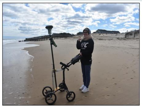
Figure 10. Student surveying a beach profile using a low-cost push cart and high grade GPS equipment. The antenna is at the top of the pole.
