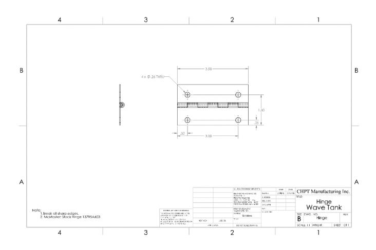
*Figure A22. Snapshot of CAD drawing for the hinge connecting the wave paddle to the flume. A PDF version of the file is available upon request.*
