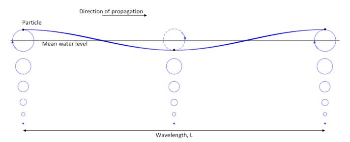
*Figure 7. Schematic showing water particle trajectories for a sinusoidal wave and how they decay with depth.*
