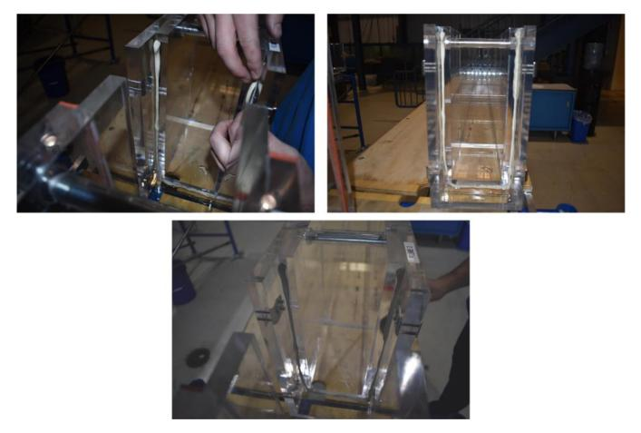
*Figure A8. Pictures showing placement of plumber's putty on the interior flume face.*
