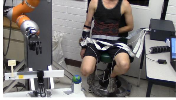
Fig. 3. Robot control setup including the sEMG systems, LWR 4, iLIMB, and three target objects to grasp and move to the bin.
