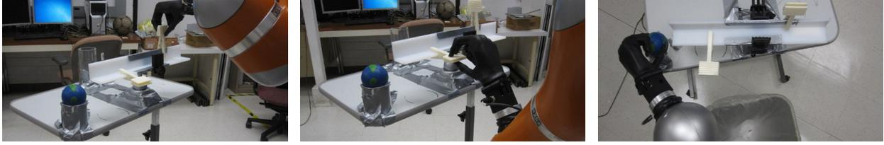
Fig. 5. Subtask sequence for the robot interface. The robot hand is controlled to grasp two clothespins and a ball. Each object is arranged such that the hand must change both position and orientation to grasp the object. The object is then placed into the bin below the table. The order in which these tasks are completed is determined by each subject. The clothespins must be grasped as shown in the images to successfully complete the task.
