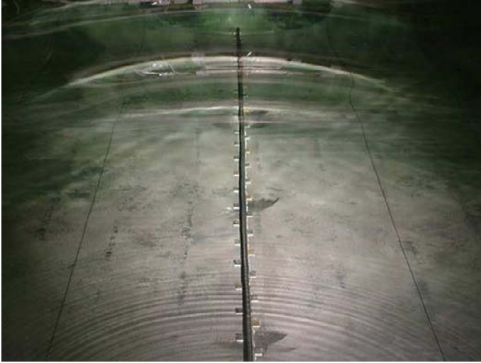
Fig. 11. Example of experimental surface elevations generated for d = 0.12 m at t \simeq t_0 . Note, the submerged model slide is visible underwater at the top of the picture.
