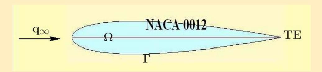
The NACA airfoils are airfoil shapes for aircraft wings developed by the National Advisory Committee for Aeronautics (NACC). The shape of the NACA airfoils is described using a 4-digit series following the word NACA. The formula for the shape of a NACA 00xx foil, with xx being replaced by the percentage of thickness to chord.
