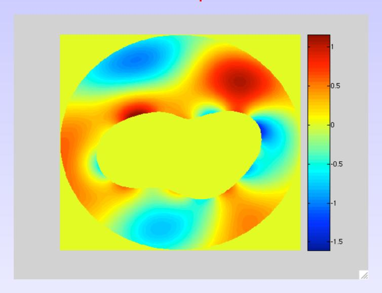
Acoustic source: Plane incident wave from left  $ka = 1.0, R = 0.95\lambda$
