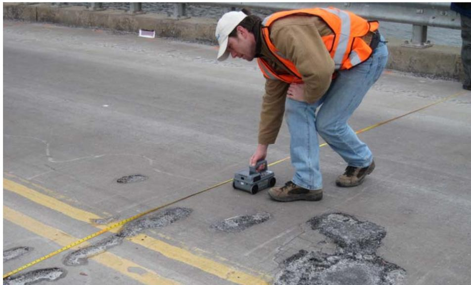
**Fig. 2.** Scanning of a concrete bridge deck using hand-held ground penetrating radar (GPR) instrument.
