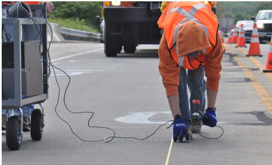
**Fig. 3.** Impulse response (IR) testing of a concrete bridge deck.
