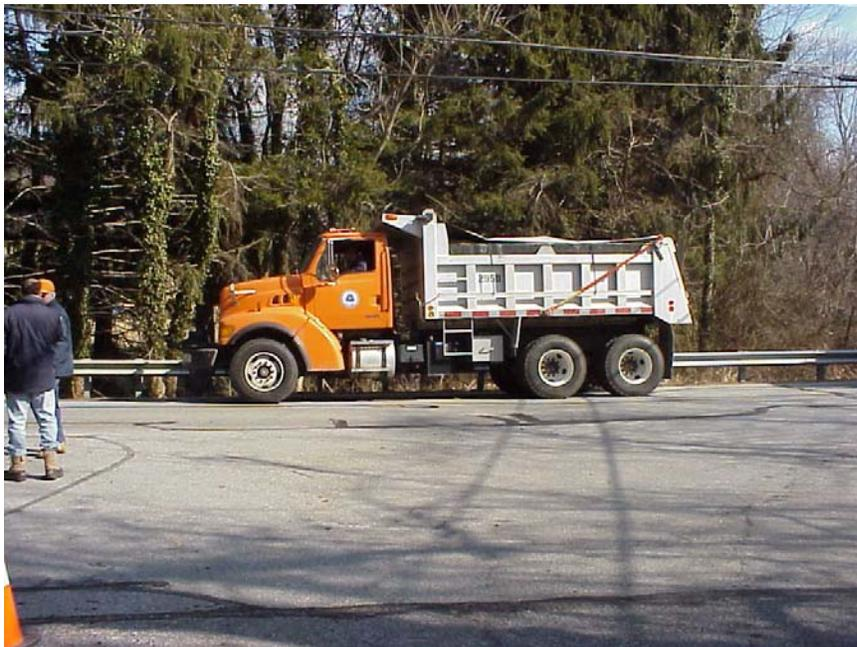
**Photograph 4. DeIDOT Truck Used in the Experimental Load Test.**
