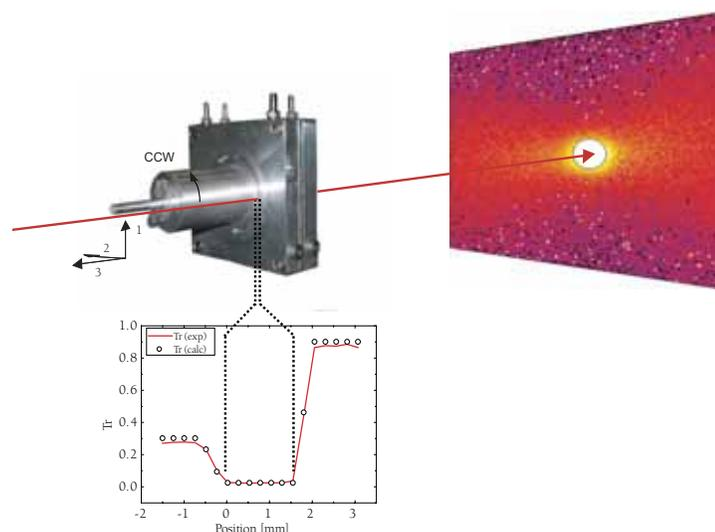
FIGURE 1: Illustration of the **1-2** plane shear cell in the neutron beam allowing for gap-resolved studies. The graph shows the recorded and predicted transmission as a function of beam position along the **2** axis using the 0.6 mm slit.
