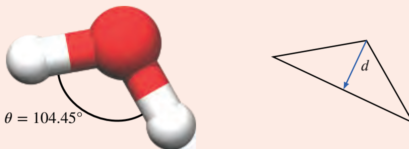
FIGURE 1.1.2 The geometry of a water molecule. \theta is the angle between the two O–H bonds. The direction of the molecular dipole ( d ) is shown on the right.
