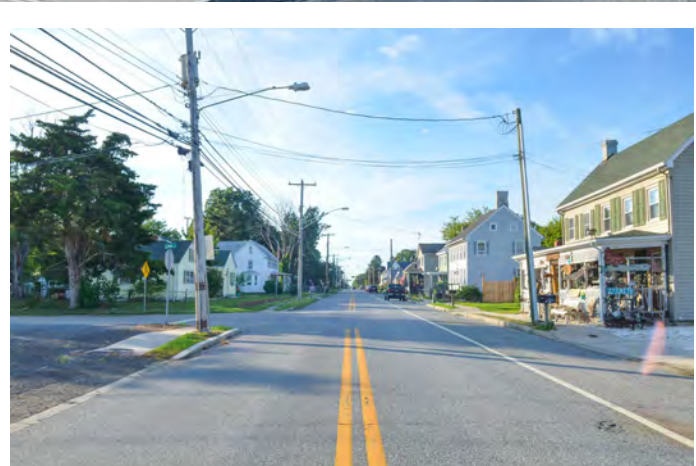
This is a photo rendering of Main Street with the addition of street banners and a painted parking lane, both treatments are designed to visually constrict the roadway and slow traffic.
