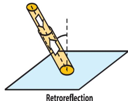
night. That is why sign sheeting materials are designed to be retroreflective, wherein the light source (in this case, from our headlights) is reflected back along the same axis with a minimum of scattering. This allows the sign to be located safely out of the line of travel and yet be visible at night.
