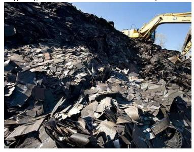
provide an economic benefit and even provide improved pavement performance by way of improved rut resistance and material stability. However, the harder asphalt cement may increase low temperature fatigue and contribute to cracking.
